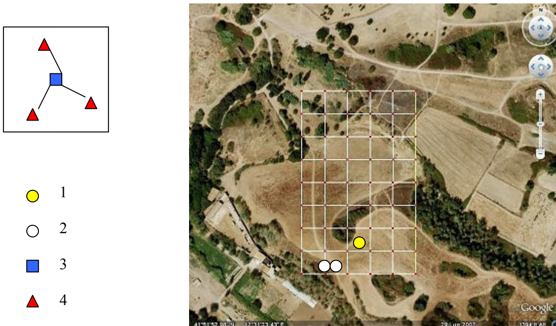
Figure 4. Location of sampling areas (A) and array of sampling stations in each area for replicate soil permeability and soil gas sampling with different approaches (B). Numbers. 1 and 2 stand for permanent and mobile sampling areas, respectively; 3 is the inner station where the Durridge approach was tested and 4 are the sites where radon v.o.s system for soil radon monitoring and soil permeability measurements was applied.
